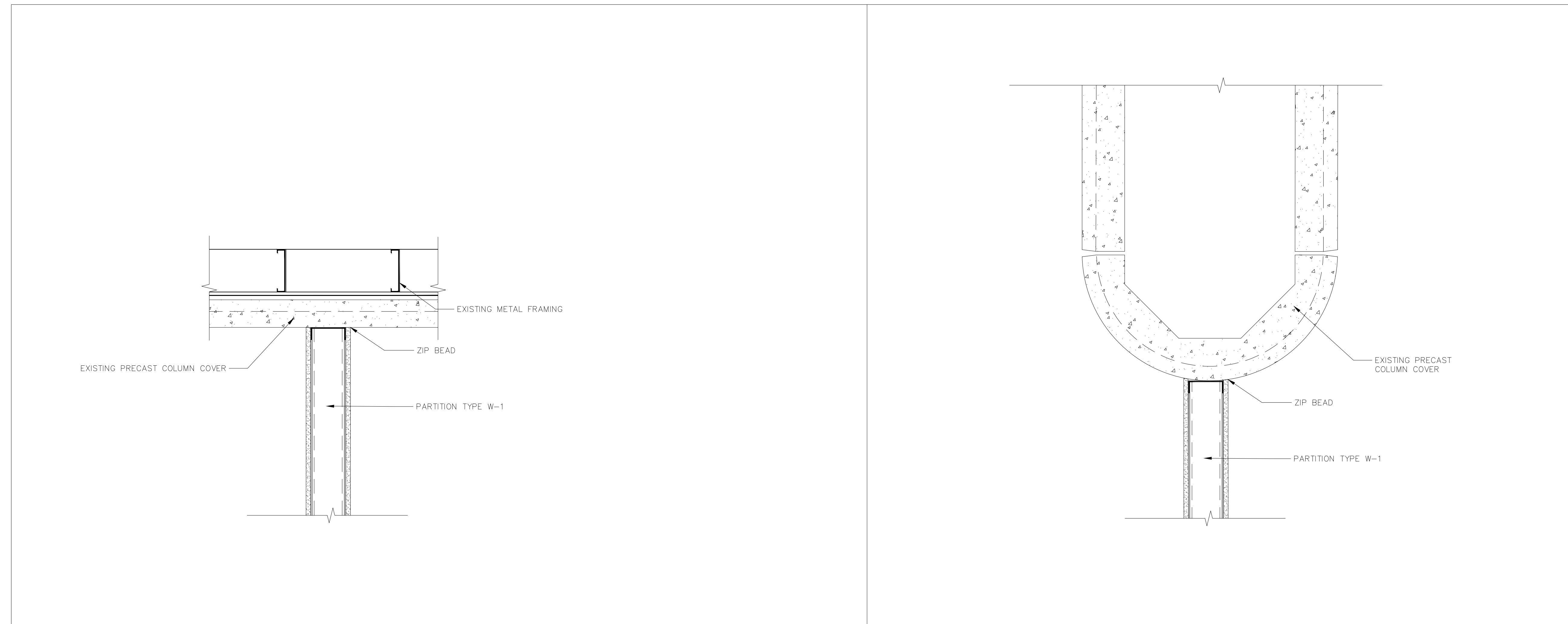
1 PLAN DETAIL - PARTITION TO FLAT PRE-CAST 2 PLAN DETAIL - PARTITION TO CURVED PRE-CAST
