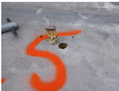
Visual image of wet core cut
