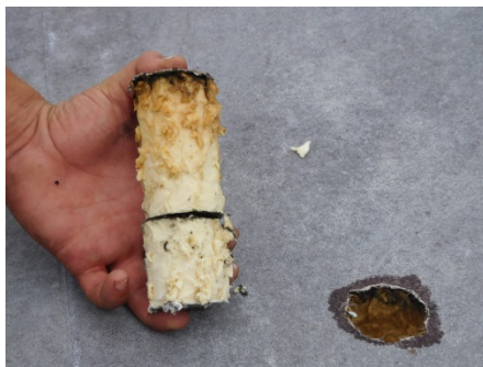
Visual image of wet core cut
