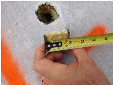
Visual image of wet core cut
