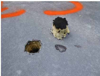
Visual image of wet core cut
