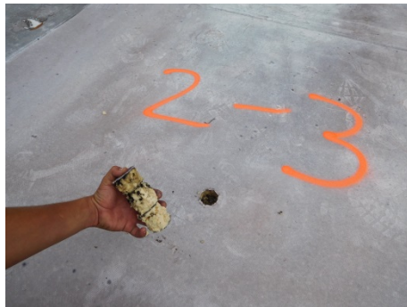
Visual image of wet core cut
