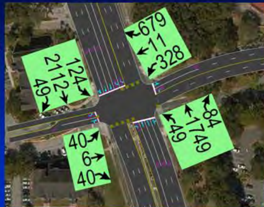
Circular Green for Thru with FYA for RT & Yield to Ped Sign
