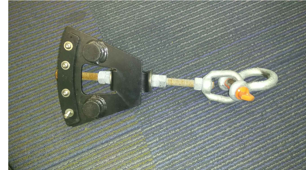
BOTTOM VIEW OF SAIL TENSIONER UNIT WITH QUICK RELEASE
