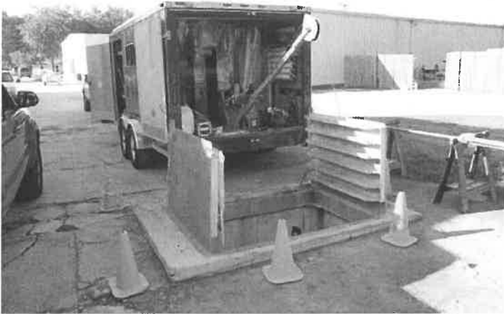
13. View of geophysical logging equipment during caliper logging
