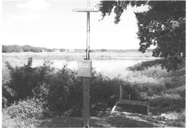
04. Inflow area located at lake, with lake level monitoring station installed by SJRWMD
