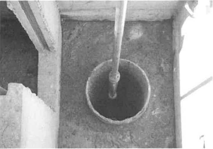
12. View of caliper logging.
