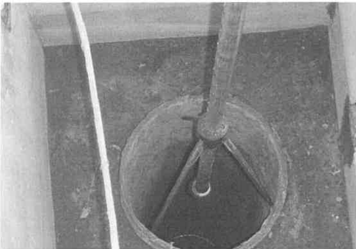
15. View of caliper tool in well following logging
