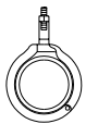
ADJ. SWIVEL PIPE RING SPLIT RING TYPE OR SOLID RING TYPE TYPE-6
