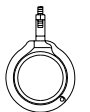
ADJ. SWIVEL PIPE RING SPLIT RING TYPE OR SOLID RING TYPE TYPE-6
